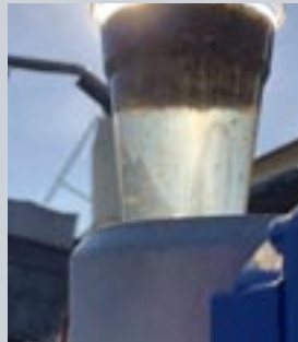
Wastewater treated with VernEx P. Sludge floats
