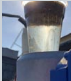
Wastewater treated with VernEx P. Sludge floats
